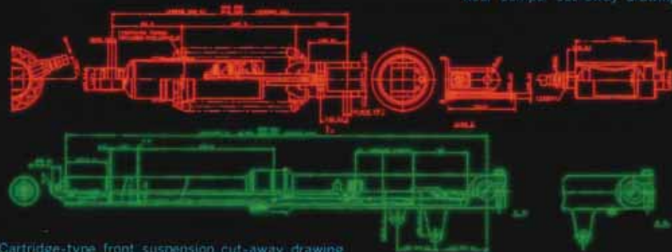
Cartridge-type front suspension cut-away drawing
