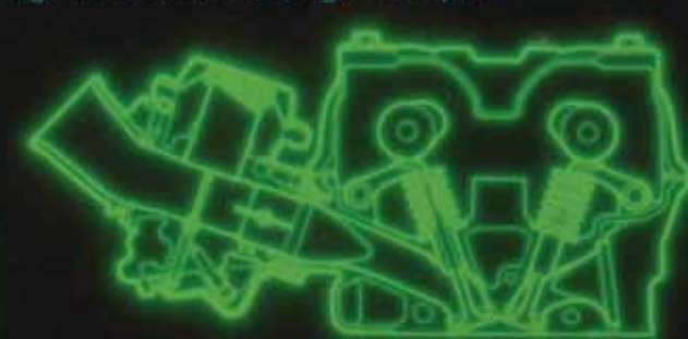
Big bore carburetor and straight intake port
